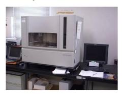
The ABI PRISM® 3730 Genetic Analyzer is a 96 capillary electrophoresis system. It is capable of performing sequencing analysis and fragment analysis, and can be used in various applications by using different lengths of capillaries. The ABI PRISM® 3130 Genetic Analyzer is a 16 capillary system and is capable of performing fragment analysis using Gene Mapper software.
